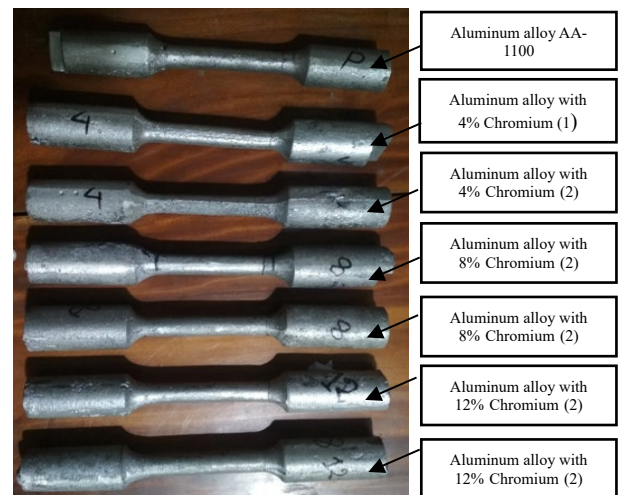
Fig. 3: Fabricated Specimen for Tensile Test
